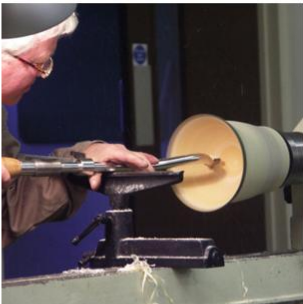
Shear scraping the inside
